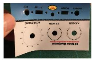
Note that the decal has overlap on all four sides. Lay the front panel face down on a clean firm surface like a cutting board or firm piece of cardboard. Use the hobby knife to trim off the overlapping sides of the decal. Use the edges of the front panel wood as a guide.
