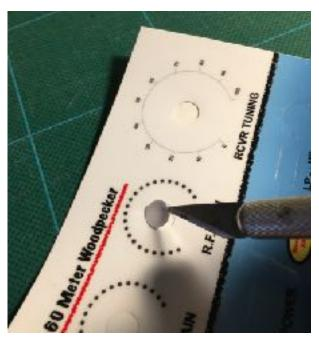
Once all the holes have been removed, the decal backing must be peeled off of the back of the decal. Carefully line up the holes with the cut out holes in the front panel wood.
