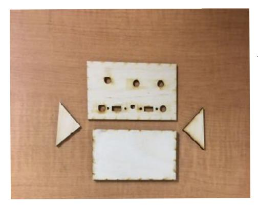
The joint may be glued to the sheet of paper. If so, gently peel the paper away. Any remaining paper should be sanded away with fine sand paper before painting.
