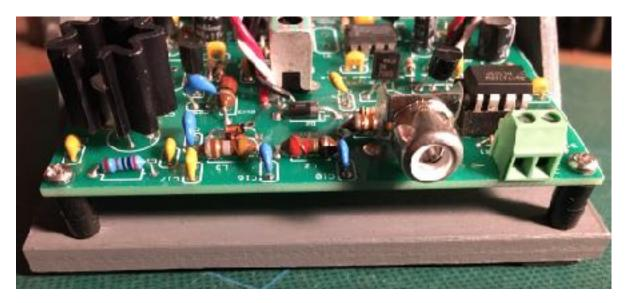
From the top of the circuit board, drill a 1/16 inch mounting hole using the corner mounting holes in the circuit board as a guide. It will not matter if the drill bit goes all the way through the wood.
