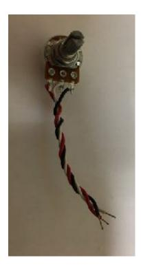
Prepare R.F. Attenuation pot with three 2.5 inch (red, white and black) wires as shown. Strip 3/8 inch of insulation from each end. Make good mechanical connections before soldering. Then twist the wires together as shown.
