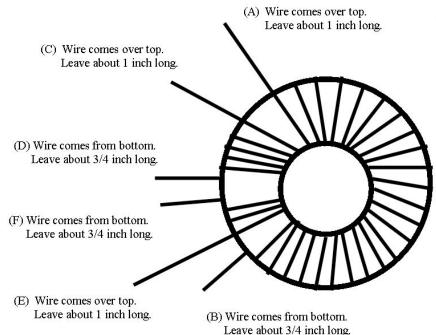
Winding #1: 24 turns, clockwise from top at (A) ending at bottom of toroid at (B).
