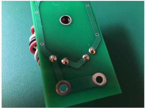
Cut soldered wires close to the board.
