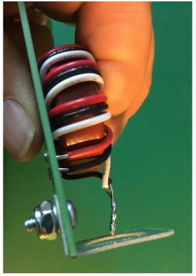
Mount the coax connector to the bracket. First, using pliers, bend the solder tab on the lock washer about 90 degrees. Then place the lock washer on the coax connector as shown.
