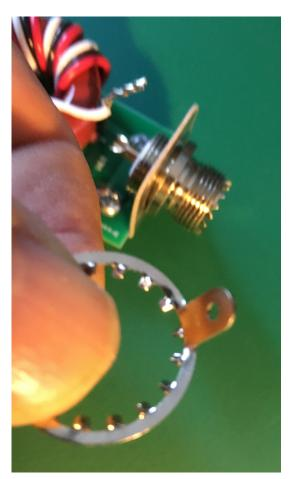
Turn the lock washer so that the solder tab is against the board. Tighten the coax connector nut tight using wide pliers or a wrench.
