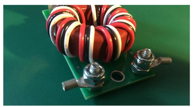
On each side, place a lock washer, plain nut, ring terminal and nylon locking nut in that order.
