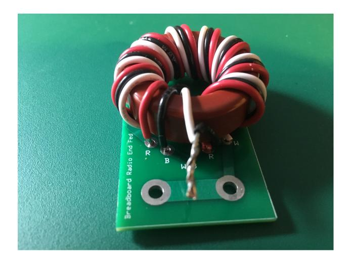
Place the remaining four (4) stripped wires into the color coded holes (red "R", black "B", red "R" and white "W".
