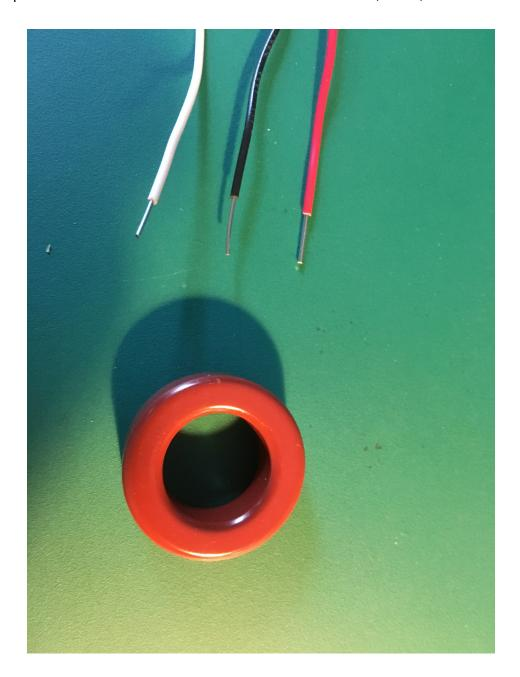
The three wires will be wrapped around the toroid together nine (9) times. Each turn should be tight and not over-lapping, but side to side (white, black, red).
