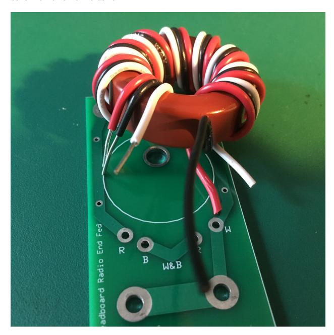
Bring the black wire straight up and bend forward at the top of the toroid as shown above. Do Not Cut Yet!
