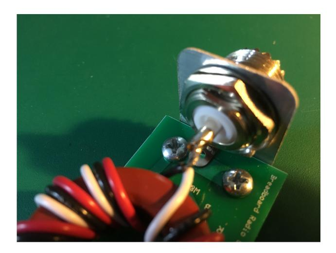
Place the twisted white and black wire into the center pin of the coax connector (trim if too long) and solder in place.
