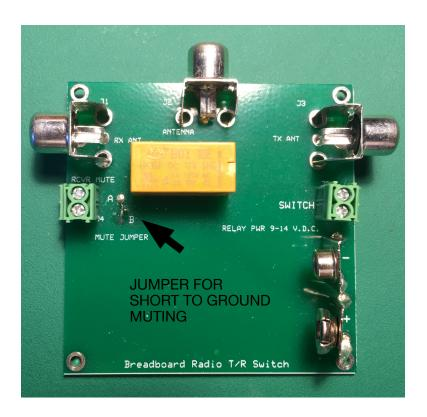
will use "open circuit" muting on transmit. If you require "short to ground" on transmit for receiver mute, you will need to solder a wire jumper between points "A" and "B" on the circuit board. Use the wire supplied and strip each end before soldering.
