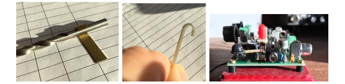
Mount the circuit board to the breadboard with four 1/2 inch brass wood screws and black 3/8th inch plastic spacers. You should have starter holes on the breadboard (Breadboard step 4.) You may need to loosen or remove the key to get the front right screw in.
