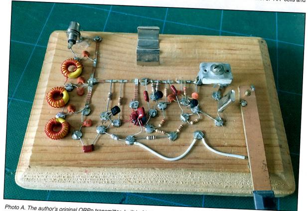
Photo A. The author's original QRPp transmitter, built in 2010 on a wooden breadboard.
